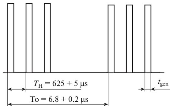
**Fig. 1.** Pulse-periodic structure of voltage pulses:  $T_c$  is carrier frequency period;  $T_e$  is the period of the envelope of the pulse repetition rate;  $t_{\text{gen}}$  is voltage pulse duration.
