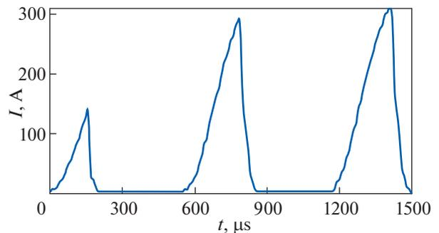
Fig. 2. Oscillogram of a series of three current pulses.
