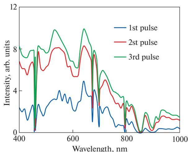
**Fig. 3.** Emission spectrum of the Cs–Hg–Xe discharge of a series of three current pulses at an electric lamp power of 1500 W.
